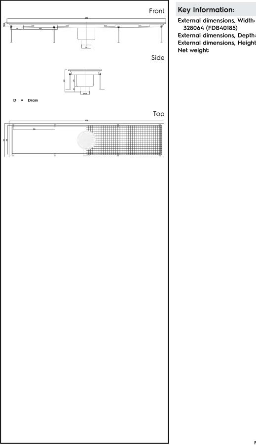
1850 mm External dimensions, Depth: 400 mm External dimensions, Height: 265 mm 30 kg
